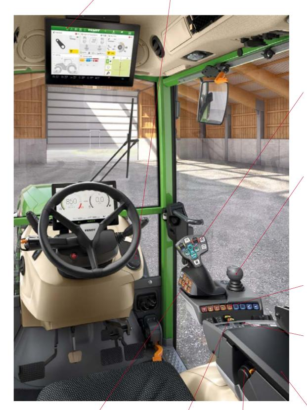
As well as the familiar clover leaf operation, the new multifunction joystick includes two controls for proportional valve control as well as four freely assignable white
