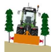
The front power lift is fully integrated and sits tight against the vehicle.
