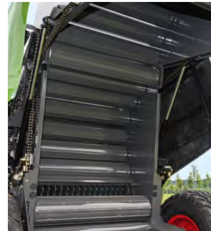
18 PowerGrip rollers will start rotation reliably ensuring even compression.
