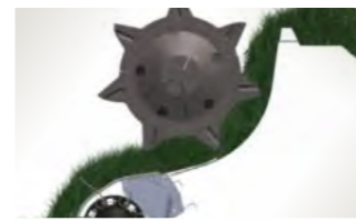
Rotor loading unit for highest throughput and uniform cutting quality
