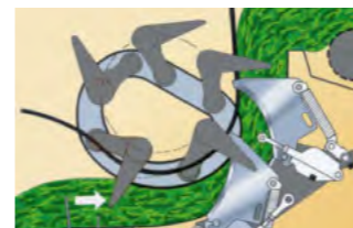
Conveyor swing unit for maximum forage protection, even with dry goods such as hay and straw.
