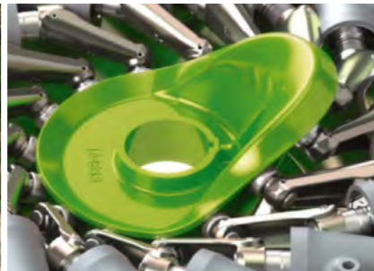
The Fendt Former cam track can be adjusted without tools and quickly, depending on the operating conditions
