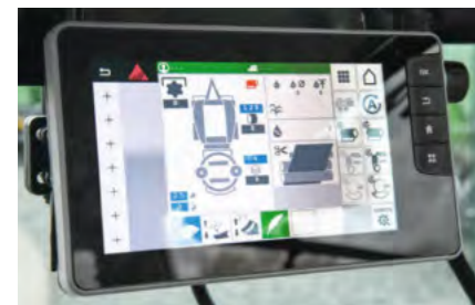
The Bale Control terminal offers you an expanded functional scope and has an ISOBUS control unit.
